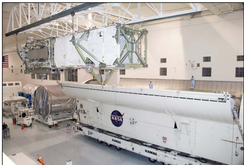
The S6 Truss Segment is loaded into the into the payload canister at the Space Station Processing Facility at NASA's Kennedy Space Center before being transferred to Launch Pad 39A for mission STS-119.
